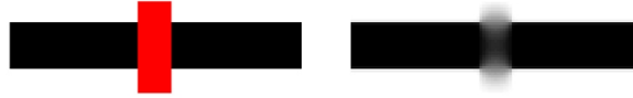
Figure 1: Left: An image of an edge with a hole. Right: the same image reconstructed using the heat equation.
